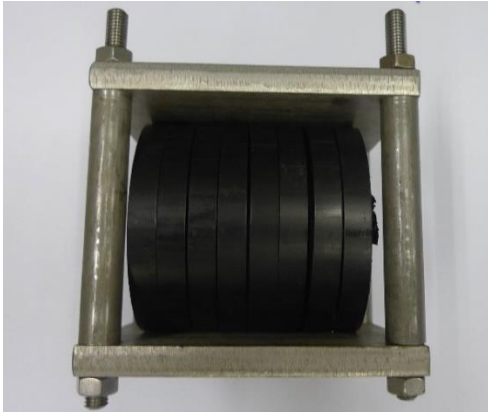
Figure 1: PE rings in a U-clamp
