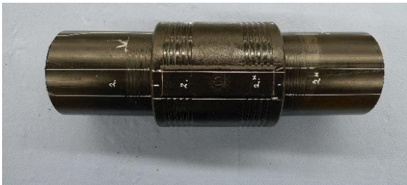
Figure 6: The electrofusion joint with the position of a tensile bar
