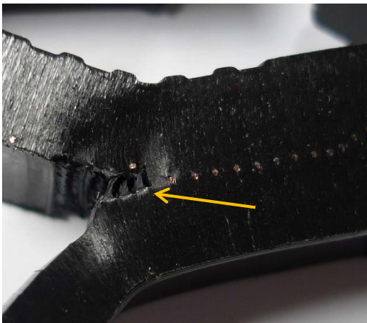
Figure 12: The yellow arrow shows the ductile failure of the joint area
