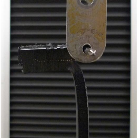
Figure 4: Execution of the peel test
