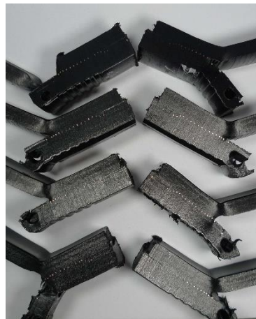
Figure 13: The visual examination showed no cavitation, which indicates a good quality joint
