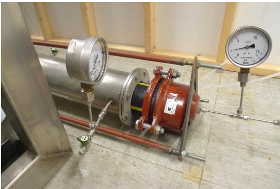
Figure 3: Permeation experimental setup in which the PE pipe (black with yellow stripes), the jacket pipe (grey) and the pressure gauge are visible
