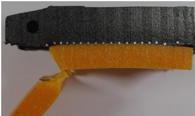
Figure 1. Failure mode IP (in the pipe wall) after the Peel test.
