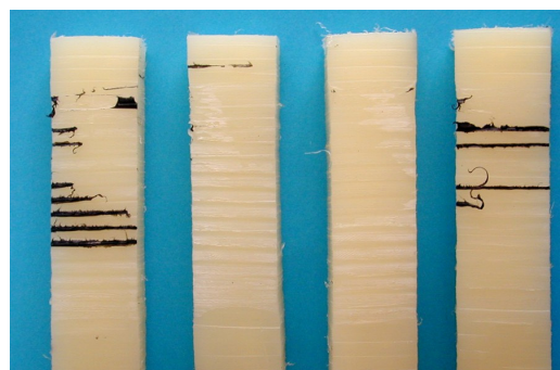
Figure 9. Test bars from an electro-fused joint in PEX pipe "D" after complete peel-off in the Slow Peel test.
