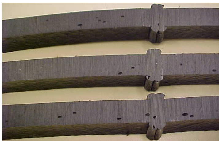
Figure 10. Test bars from a PE pipe with internal voids and a butt fused joint.
