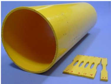
Figure 1: PVC-HI pipe with dumbbell-shaped specimens.
