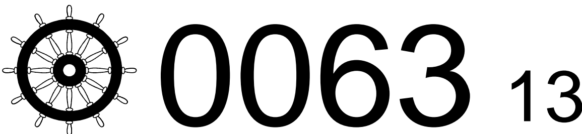
Figure 1: Marking for marine equipment approved by Kiwa and manufactured in 2013.
