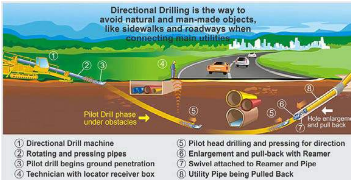
Image 6.4. Horizontal Directional Drill (HDD)
