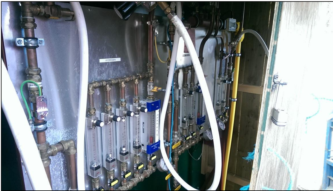
Figure 4: Test gas injection rig
