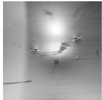
Figure 6. Inner pipe wall at the point load location of PE 2019-268 as tested in Lab 3 with Disponil® LDBS 25 at 90 °C and 4 MPa.
