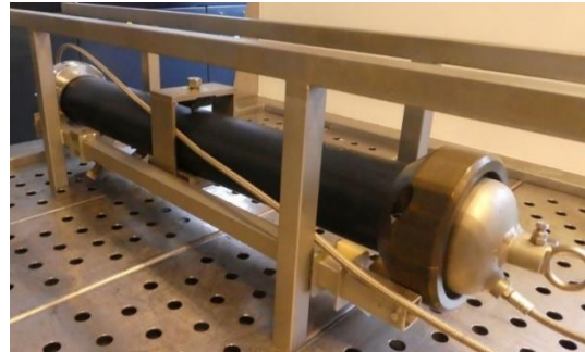
Figure 1. Left: Schematic overview of the point load test (PLT). Right: PE pipe deformed by a point load and filled with detergent solution, ready to be immersed in the water tank.
