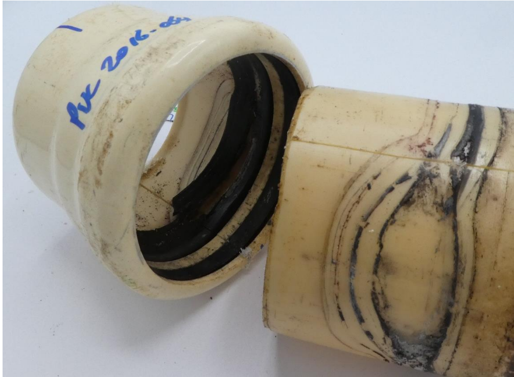
Figure 4 Disassembled PVC 2016-064 joint after testing
