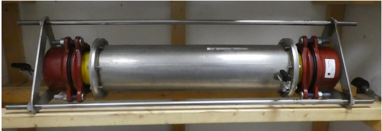
Figure 1. Sealed PVC pipe surrounded with a steel jacket pipe for the permeation measurement.
