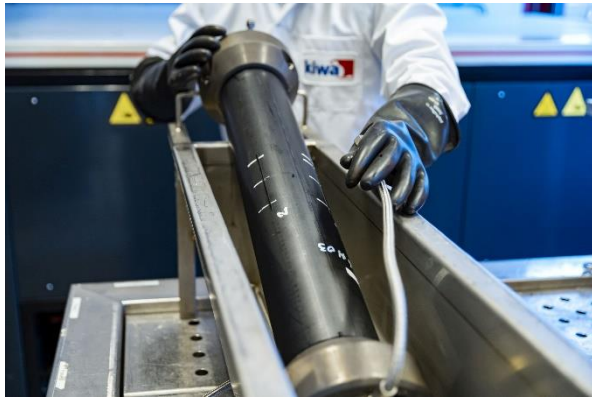
Figure 1. Placement of the test pipe in the horizontal container (still without detergent solution).
