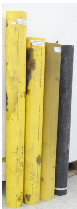
Figure 9 Four of the six tested PVC pipe segments
