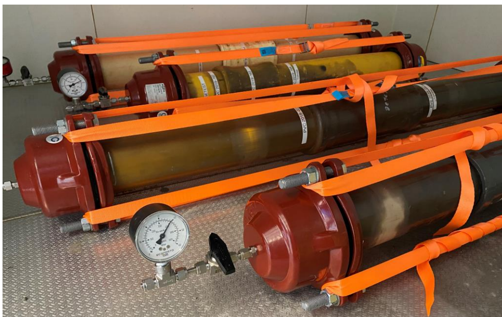
Figure 1 Ageing at 60°C of the four joints
