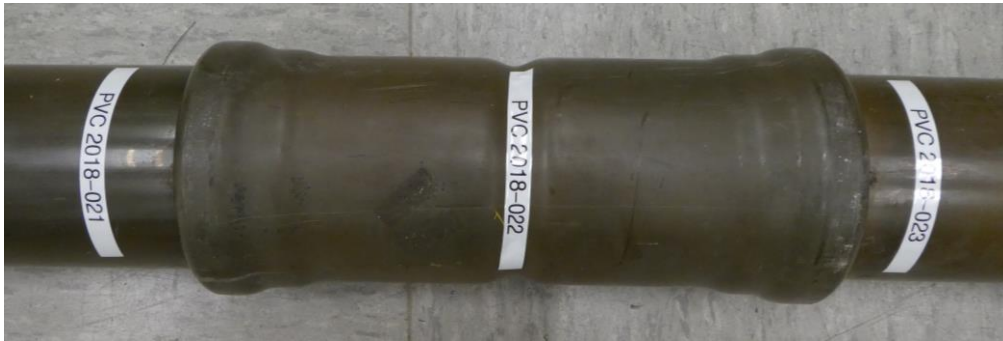
Figure 6 PVC 2018-022; PVC-Hi thermo formed coupler and PVC-Hi pipes
