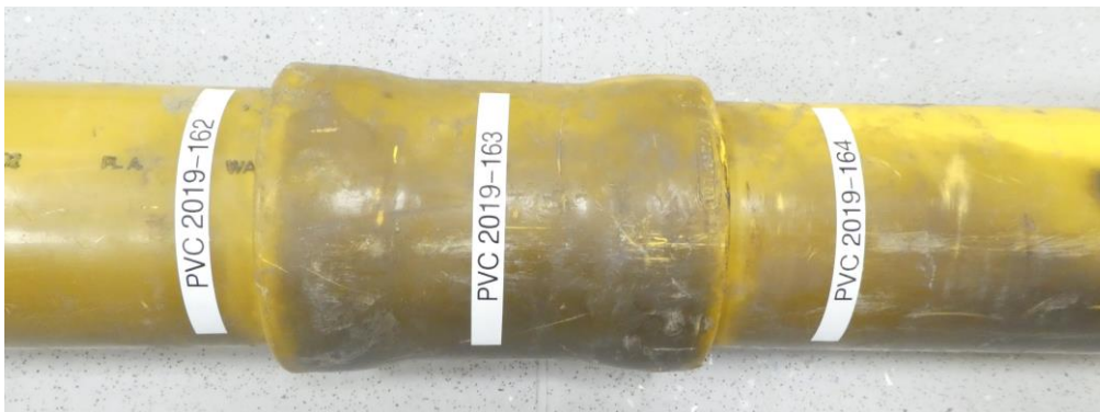
Figure 8 PVC 2019-163; PVC-Hi injection moulded coupler and PVC-Hi pipes
