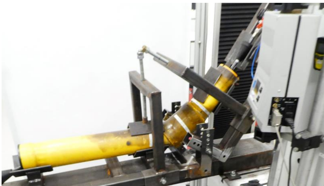
Figure 3 Angular deflection test rig (placed into a tensile test machine)
