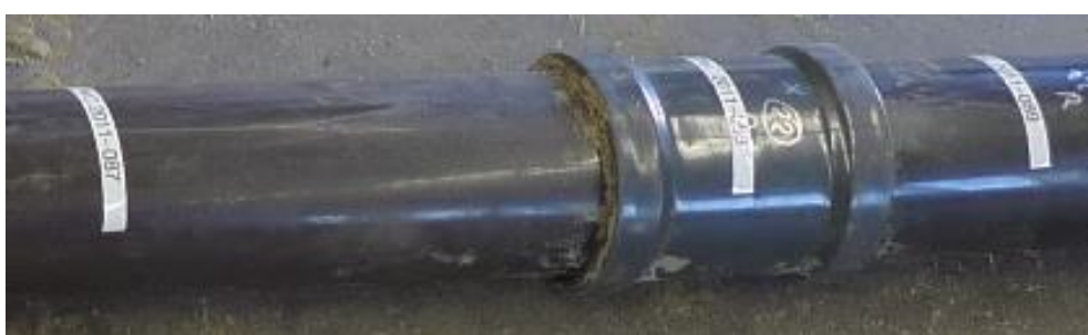
Figure 5 PVC 2011-088; PVC-U injection moulded coupler and PVC-U pipes
