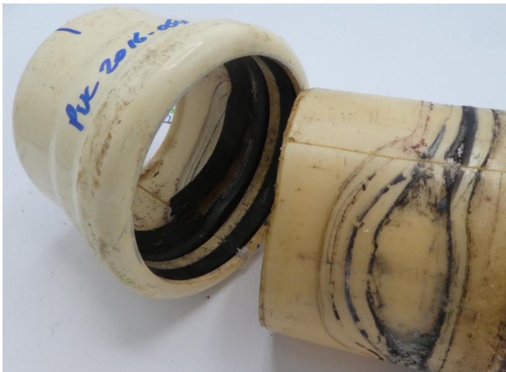
Figure 21 De-mounted joint PVC 2016-064 after testing
