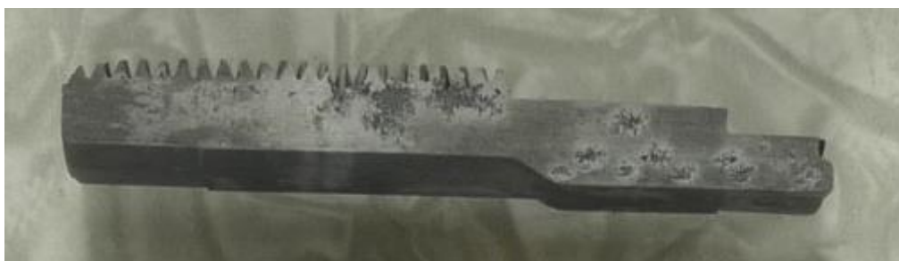
Figure 44. Pitting corrosion on machined surfaces of the corrosion sample after 19-month exposure to gas number 3.
