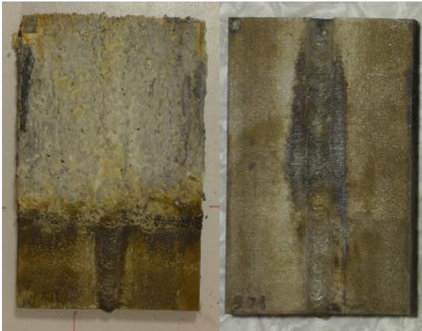
Figure 40. Corrosion sample from the experiment with gas number 1 at 8 bar(g). The exposed sample (left) shows a thick grey/white layer of ferrous hydroxides in the gas phase and the cleaned sample (right) shows preferential attack in the heat-affected zone (HAZ).
