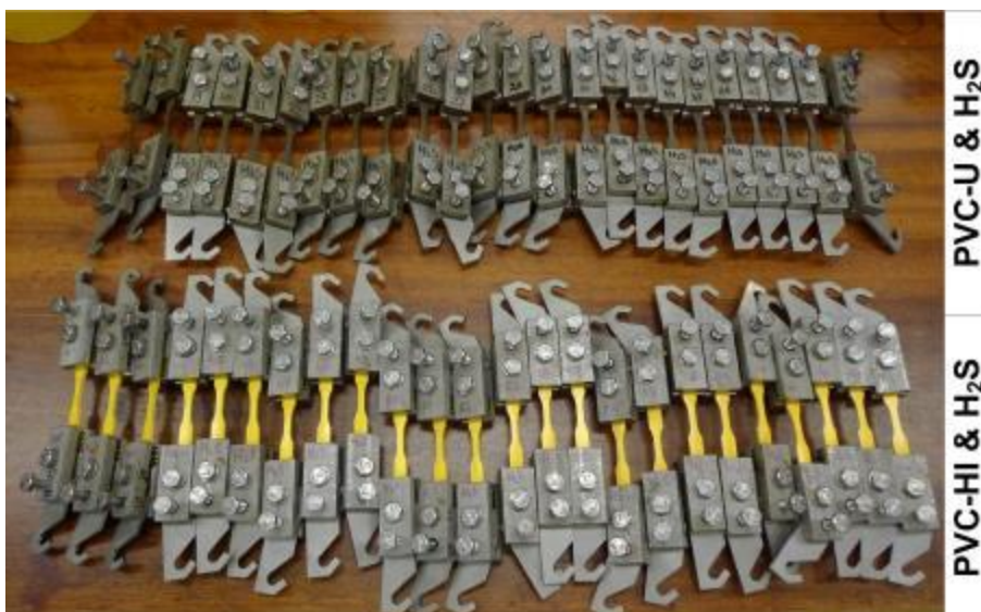
Figure 18. The dark layer after H 2 S exposure is only visible on PVC-U (top row) and not on PVC-HI (bottom row).
