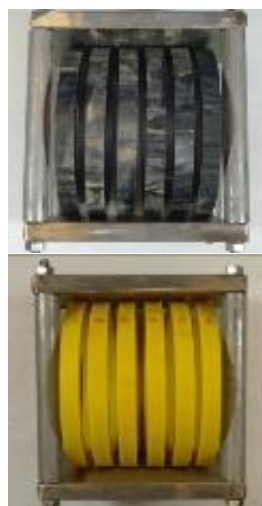
Figure 6. PE ring samples in U-clamps.
