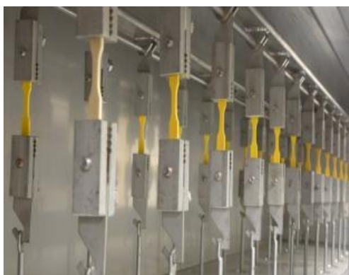
Figure 7. Constant load experiments on PVC dumbbell samples.
