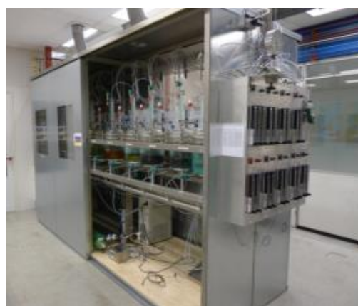
Figure 12. Complete setup for the corrosion tests.
