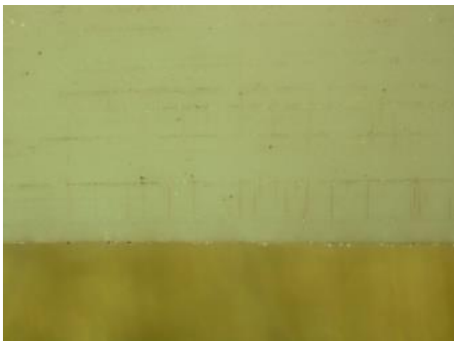
Figure 47. Crazes that have formed in PVC-U type 2 at 20 MPa that was exposed to 100% N 2 . The crazes were deliberately coloured afterwards through exposure to H 2 S without an applied stress to make them better visible.
