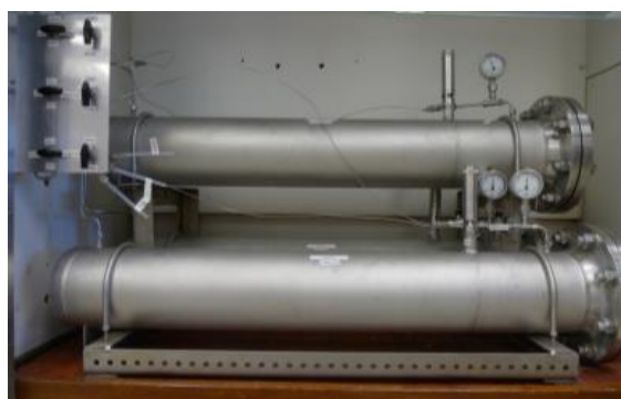
Figure 10. Full-scale test rig for 8 bar(g). Inside the test rigs, the materials are exposed to various gases.
