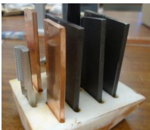
Figure 11. Metallic samples in a special PTFE holder for the corrosion test.
