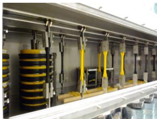
Figure 8. Constant load experiments on PE dumbbell samples and constant strain experiments on NBR samples that have been placed over oversized pipes.
